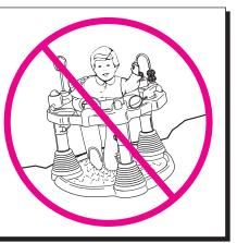
To avoid tipovers, place product on flat, level floor/ground. Adjust legs to same height so that the tray is level before placing child in product.
